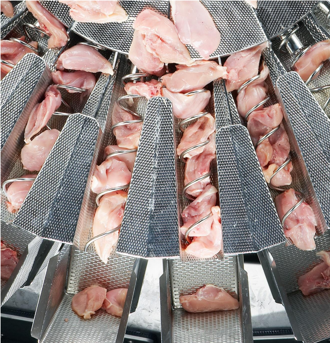
Picture 1 Cabinplant's Multihead Weigher, with the screw feeding principle, addresses irregular weights in poultry products, offering a comprehensive solution.
