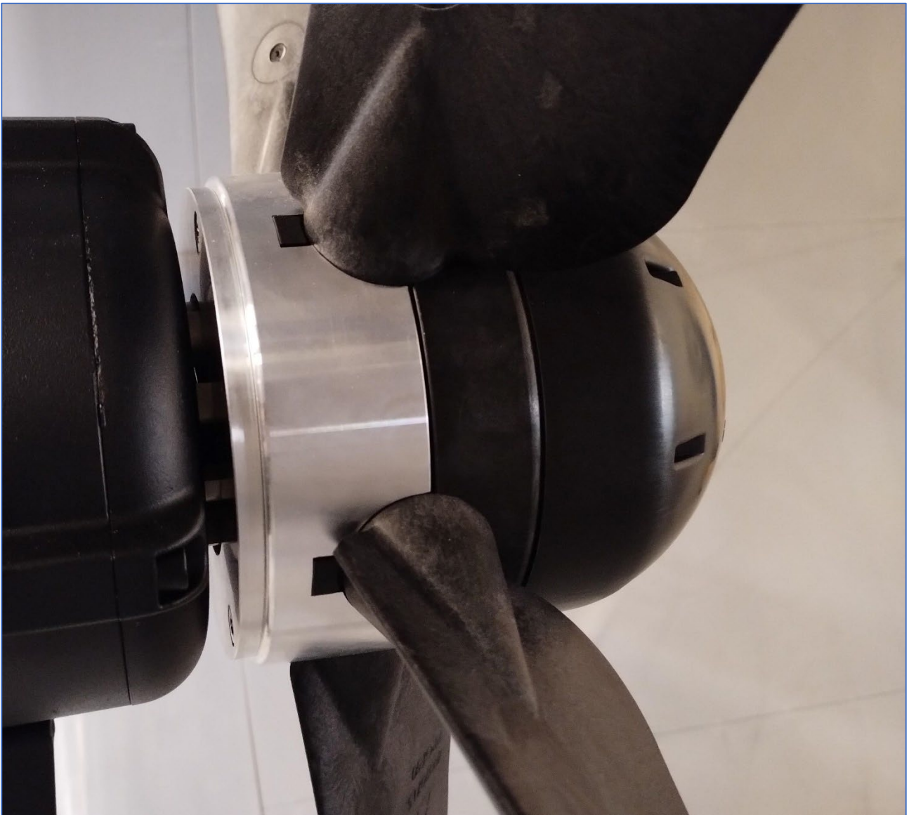
The Anti-Reverse system integrates in an aluminum back-plate mounted on the impeller hub.
