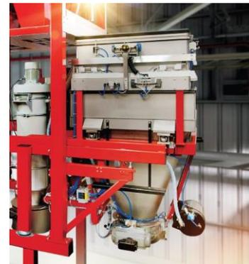
The ALFRA FCD Flexible Component Dosing System uses a dosing plateau with ALFRA Dosing Slides. Therefore it very accurately doses large and small quantities.
