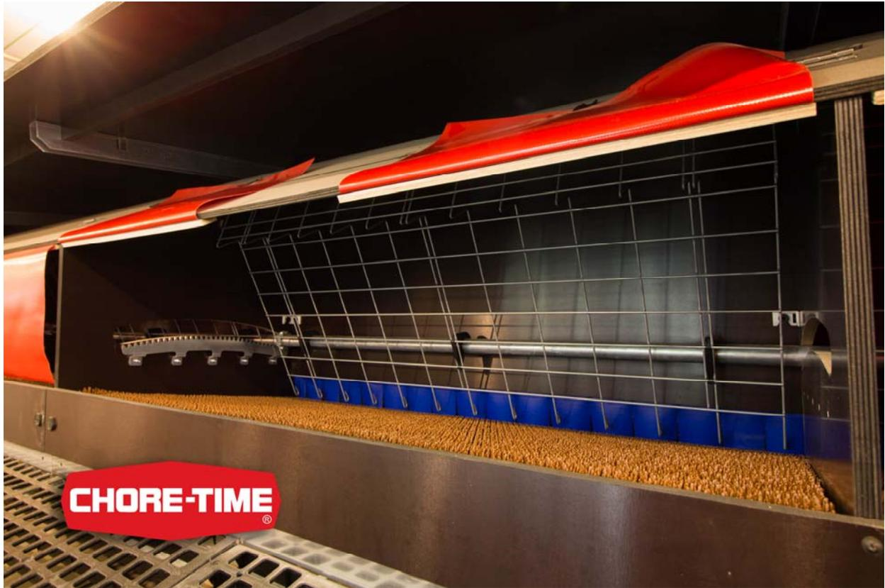
Chore-Time's Valego rack-drive expulsion system powers across nest pads for reliable, complete emptying of each nest.
