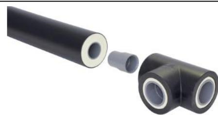
*The corrosion-free COOL-FIT® ABS Plus from GF Piping Systems is a pre-insulated plastic piping system specifically designed to meet the requirements of secondary cooling and refrigeration in food and beverage production facilities as well as others where efficient cooling is required. The '3 in 1' system incorporates: 1) a low-temperature COOL-FIT ABS carrier piping system, 2) PUR (polyurethane foam) insulation, and 3) and white or black outer jacket.*
