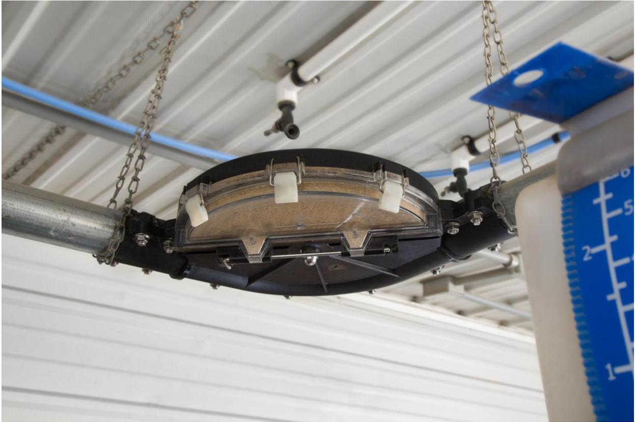
Hog Slat's E-Z Clean Corner features a transparent cleaning door, enabling quick visual inspection of accumulated feed.
