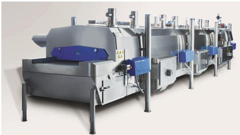
Among the technologies Linde will be presenting at IPPE 2018 is a new wave-impingement freezer which combines cryogenic gas impingement with new dual-action product agitation. The CRYOLINE® CWI CRYOWAVE™ impingement freezer offers production capacity up to 6,000 lbs. per hour.
