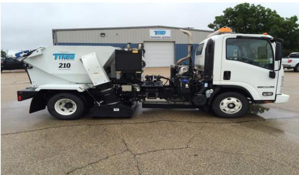
Developed at first with parking lot sweeping in mind. The Model 210 has brought the Regenerative Air System power and efficiency to a smaller version TYMCO sweeper. The Model 210 for decades has been the workhorse for sweeper contractors and property owners alike. The material and craftsmanship that goes into the larger TYMCO sweepers goes into the Model 210.
