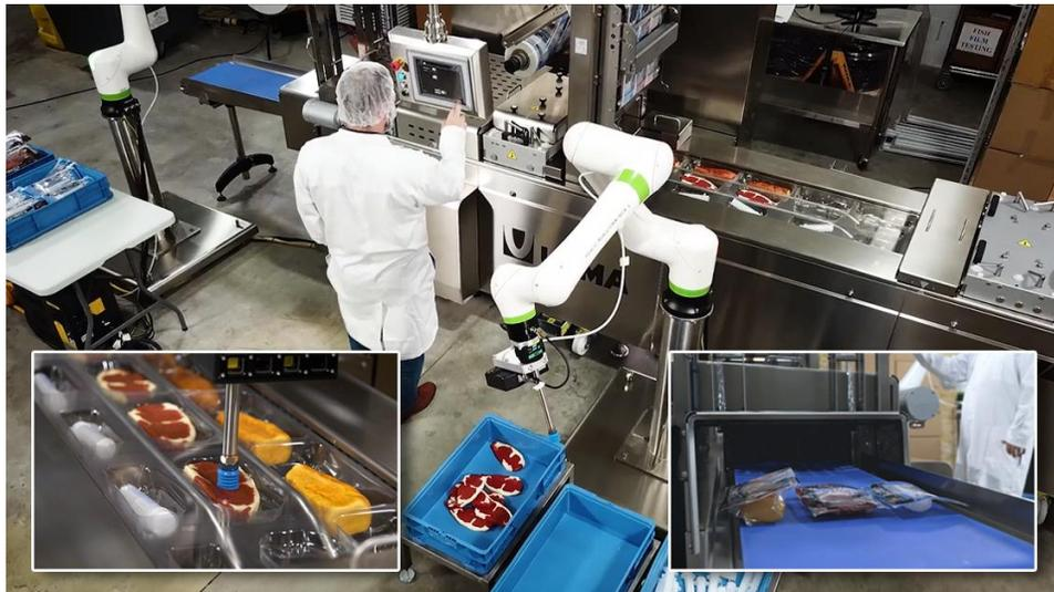
*As part of Harpak-ULMA's TFS500 smart, connected thermoforming machine demonstration, three different products are run simultaneously while leveraging FANUC America's CRX collaborative robots to load and unload the irregular sized products. The demonstration unit will be on display at PackExpo 2021 in Las Vegas, and can be viewed starting in December 2021 at PTC's Boston Seaport CXE Center, followed soon after at the company's new headquarters location in Taunton, MA. (Photo: Business Wire)*
